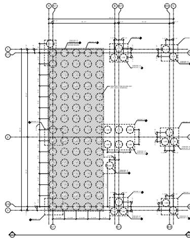
The preliminary layout of Aggregate Piers is shown to the left for the Todd Creek Waste Water Treatment Plant in Kansas City, Missouri.
